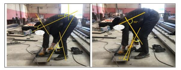
In the third stage, the connection of the main chassis is completed. The A (5) and B (2) scores for the two main chassis, joined by bolts and nuts, were matched in the C table, resulting in a score of 4 (Table 10). With the addition of the activity score, the REBA score was determined to be 5. The risk level for this task falls within the range of 4-7, indicating a medium risk level. As per the REBA guidelines, precautions should be taken to mitigate the risks associated with this posture.
