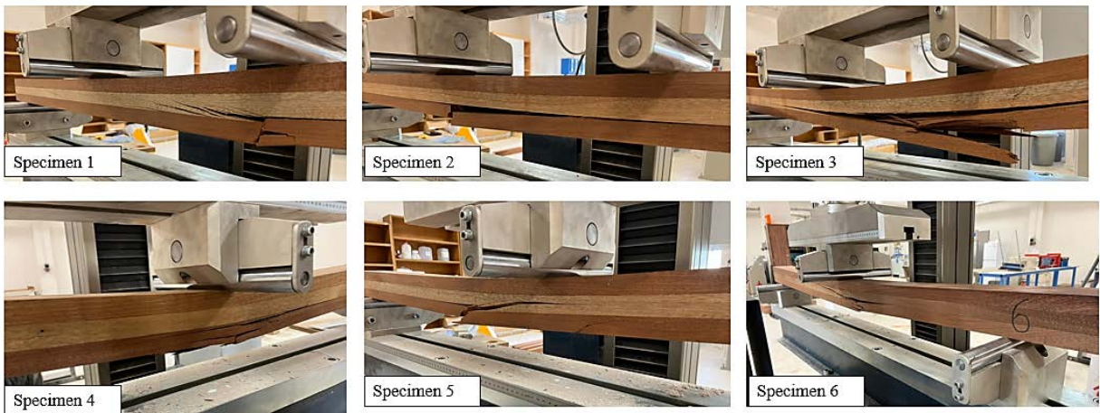
Figure 6. Failure modes of specimens.
