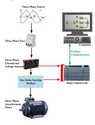
**Figure 2.** General block diagram of the system (Sistemin genel blok diyagramı)
