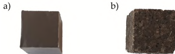
Figure 3. (a) Photograph of the composite sample produced within the scope of the study, (b) Photograph of the Sille stone
