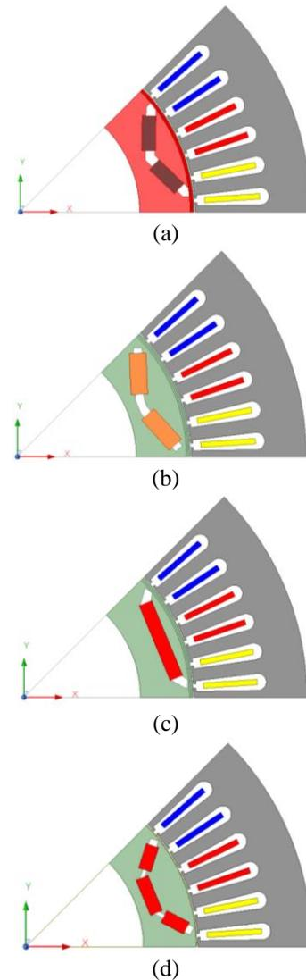
Fig.1. Final motor models (a) Reference IPMSM (b) V-shaped IPMSM (c) Flat-shaped IPMSM (d) U-shaped IPMSM
