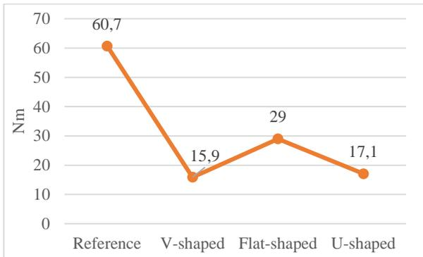
Fig.3. Torque ripple comparison chart
