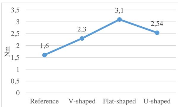
Fig.5. Cogging torque comparison chart
