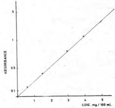
Fig. 2. Salicylic acid standard calibration curve.
