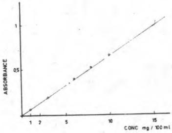
Fig. 1. Aspirin standard calibration curve.
