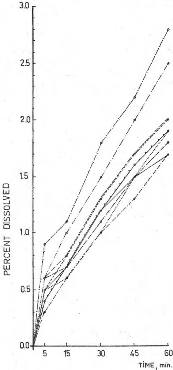
Fig. 5 - Cumulative percent of Salicylic acid dissolved from Aspirin plain tablets manufactured in the U.S.A (—); in ENGLAND (— — —); in IRAN (.....); in W. GERMANY (---); in SWITZERLAND (— · — ·); in TURKEY I (— · — · —); in BELGIUM (— · — · —); in TURKEY II (— · —); in FRANCE (— · — ·)
