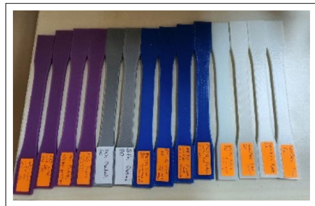
Figure 9. Image of the some printed specimens before tensile test.
