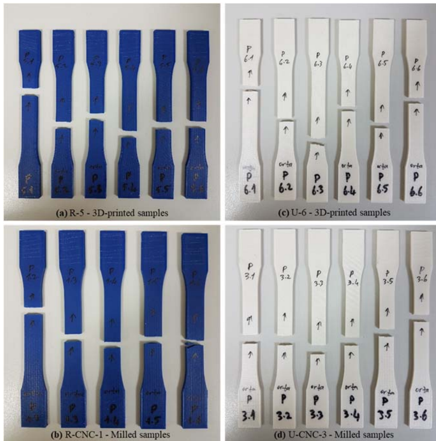
Figure 5. Images of broken samples
