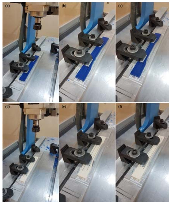
Figure 2. Converting rectangular samples into dog-bone shape with CNC milling
