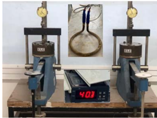
Figure 2. Consolidation test equipment at room temperature and 40°C
