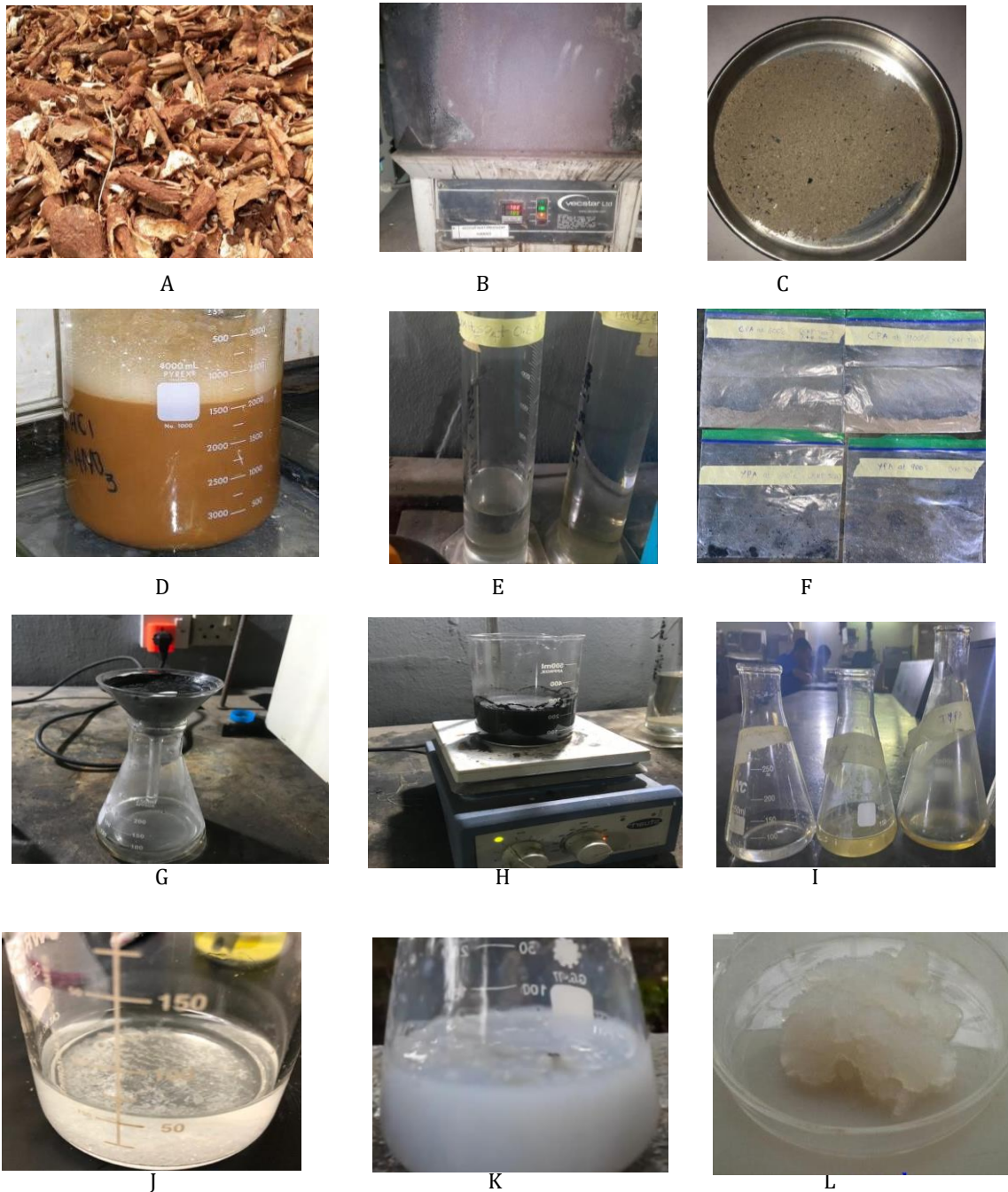
Fig. 1 Pictures showing (A) Washed and dried Cassava Periderm, (B) Calcination Of Periderm to ash in Furnace, (C) Silica ash from periderm, (D) Preparation of reagent, (E) Washing of silica ash in acid, (F) Labeled purified silica ash, (G) Leaching of Silica Ash in Alkaline Solution, (H) Filtration of \text{Na}_2\text{SiO}_3 solution, (I) Filtrates of \text{Na}_2\text{SiO}_3 , (J) Titration and precipitation of \text{Na}_2\text{SiO}_3 , (K) Aging of silica gel, and (L) Synthesized aqua silica
