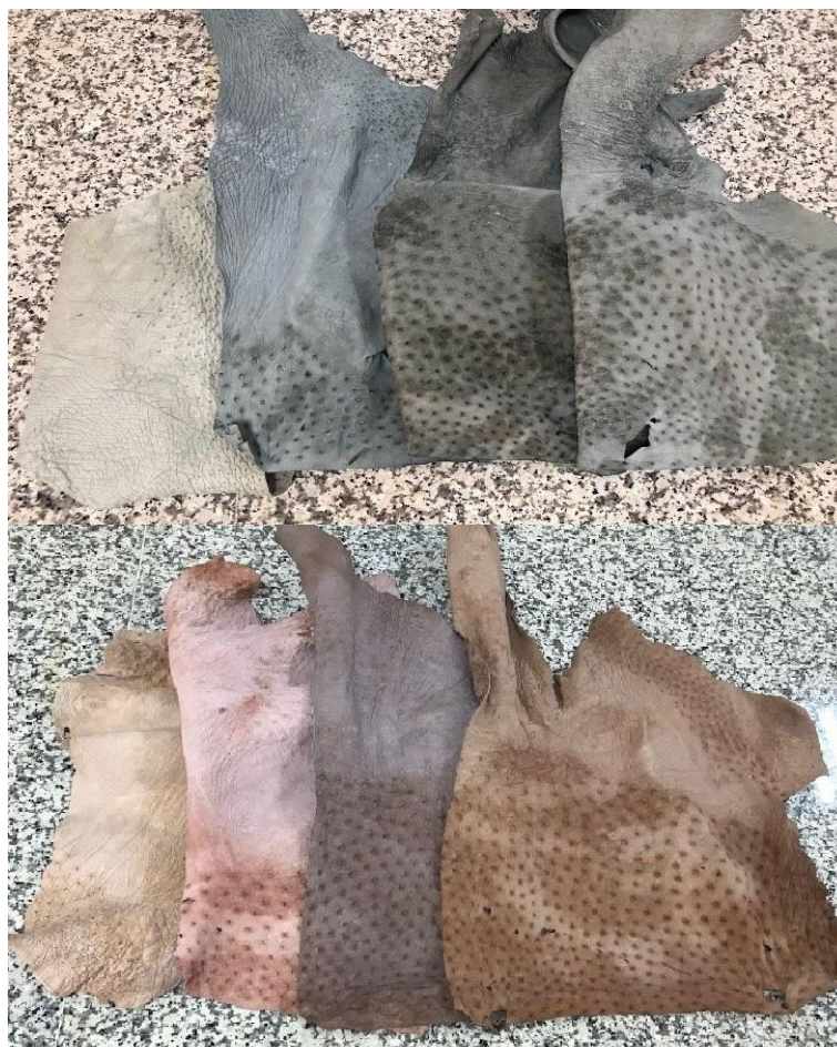
Figure 6. Dyed ostrich leathers (Top row: Chrome-tanned; bottom row: vegetable-tanned, in order from left to right according to the codes)
