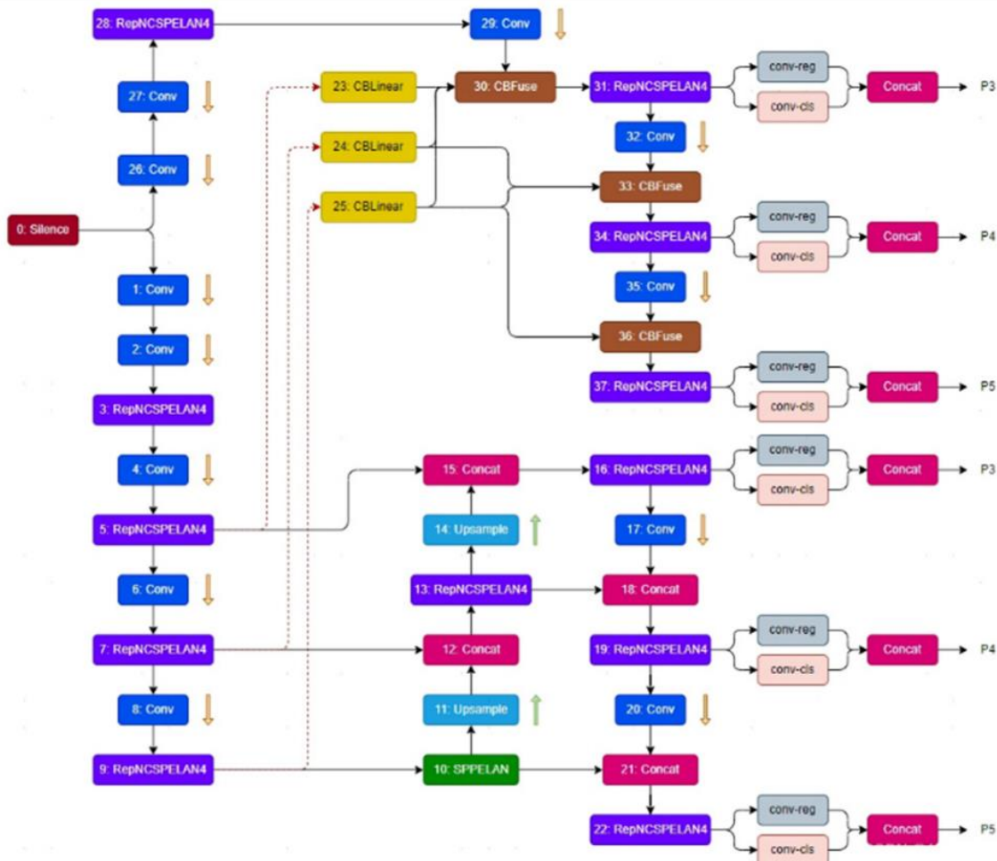
Figure 3: YOLOv9 architecture (Wang, 2024)
