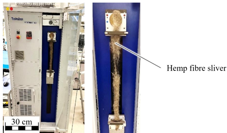
Fig. 2. Test setup and realisation of the adhesion-slip test
