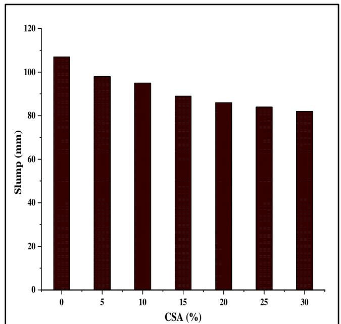
**Figure 5.** Workability of CSA in concrete
