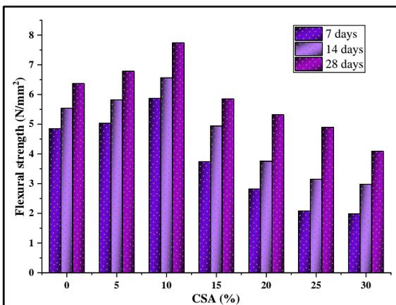
Figure 9. Flexural strength test results
