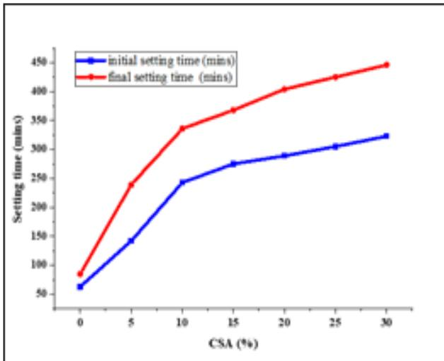
**Figure 4.** Initial and final setting time of CSA in concrete
