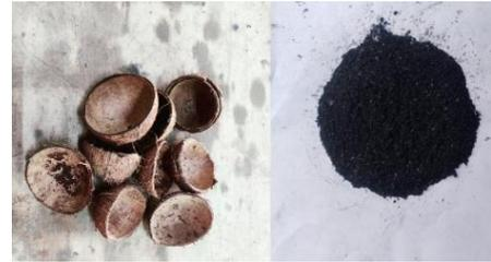
**Figure 3.** Coconut shell into CSA
