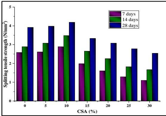
Figure 8. Splitting tensile test results
