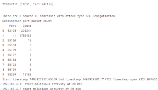
Fig. 11. SSL Renegotiation Attack Summary: Packet Distribution, Timestamp, and Source IP Details.
