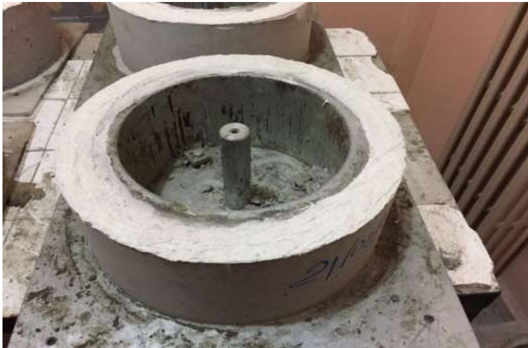
Figure 3. Rest ring shrinkage test.
