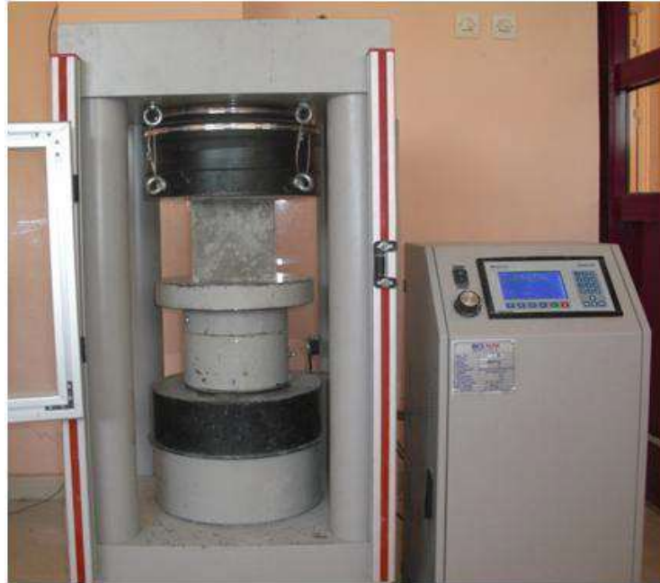
Figure 1. Compressive strength test.
