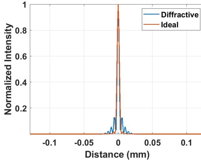
c) Comparison of the 1D intensity distributions of the diffractive lens and its equivalent ideal lens.
