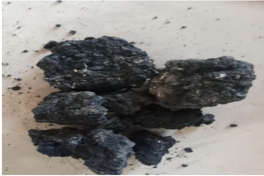
Figure 1. Crumbs of RAP in raw state
