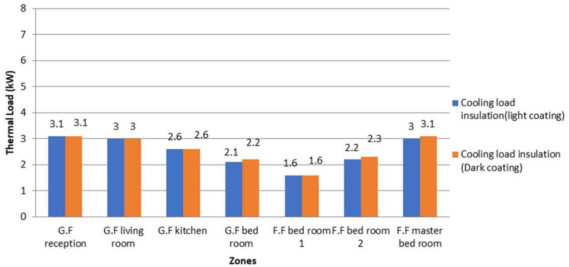
Figure 5. Cooling load insulation (light coating vs. dark coating)
