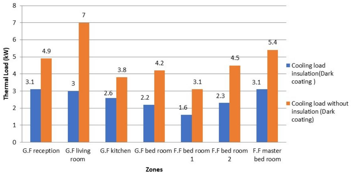
Figure 4. Cooling load with insulation vs. cooling load without insulation (dark coating)
