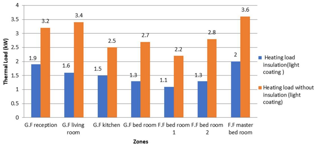
Figure 7. Heating load insulation vs. heating load without insulation (light coating)
