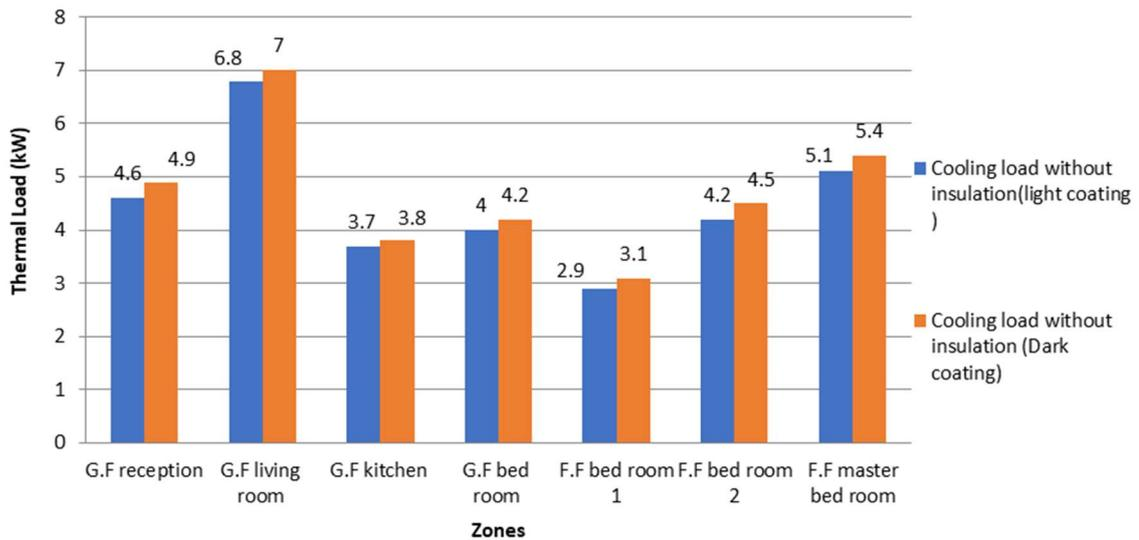
Figure 6. Cooling load without insulation (light coating vs. dark coating)
