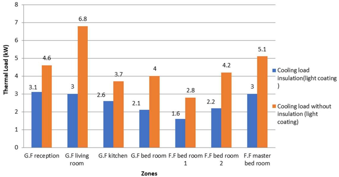
Figure 3. Cooling load insulation vs. cooling load without insulation (light coating)
