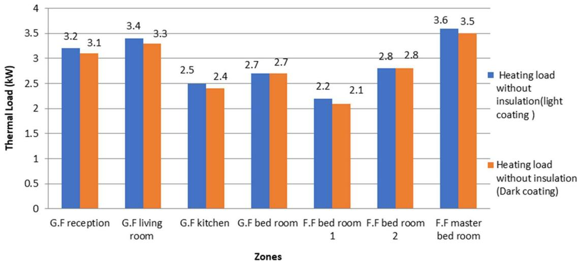
Figure 10. Heating load without insulation (light coating vs. dark coating)
