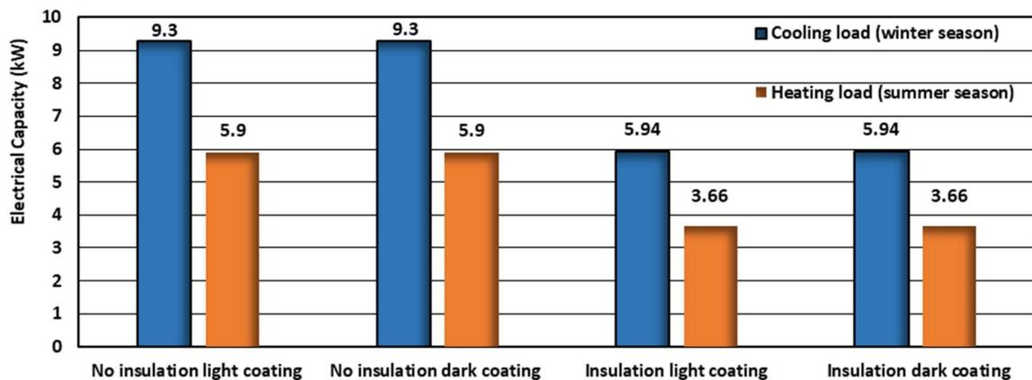
Figure 12. Electrical capacity for (cooling and heating load) in summer and winter seasons
