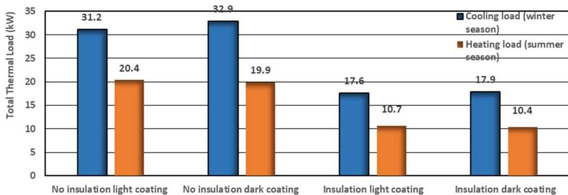
Figure 11. Total heating and cooling load (light coating vs. dark coating)
