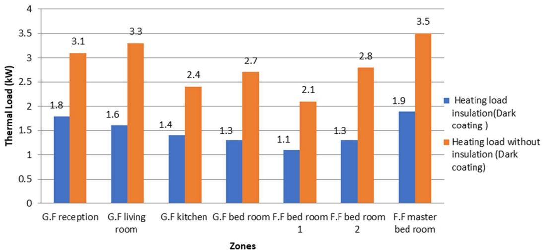
Figure 8. Heating load insulation vs. heating load without insulation (dark coating)
