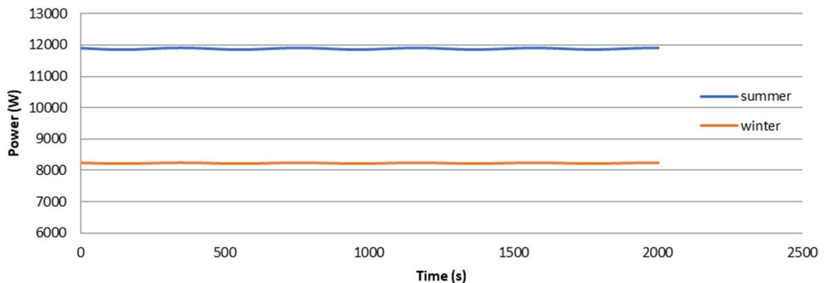
Figure 13. The output power of solar panel system
