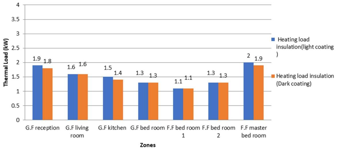
Figure 9. Heating load with insulation (light coating vs. dark coating)
