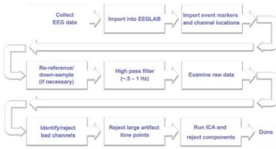
**Figure 7.** Pre-Processing pipeline in EEGLab (Delorme, 2019)
