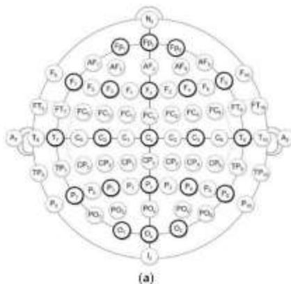
**Figure 2.** The 10-20 electrode placement system
