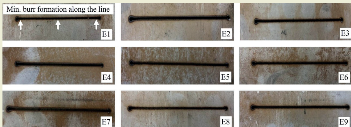
Figure 12. Bottom surface burr formation after cutting on a 8 mm thick plate
