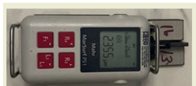
Figure 6. MarSurf PS1 surface roughness measuring device
