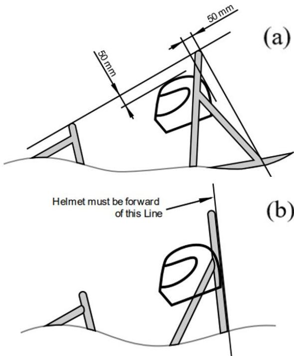
Figure 4. Measurements of driver's position(a), Positioning of the driver (b) [71]
