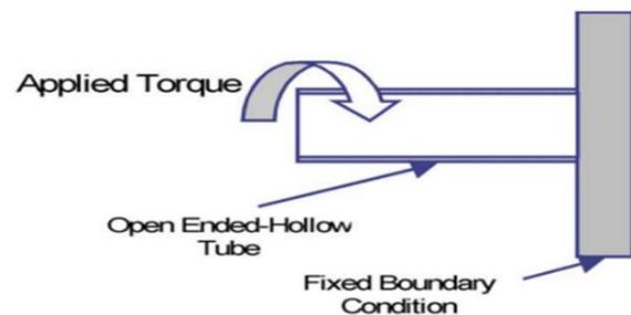
Figure 15. Torsion Tube This concept, when applied to the real car frame would look like follows [112]
