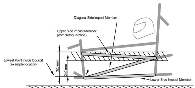
Figure 6. Position and placement of side impact structures [71]
