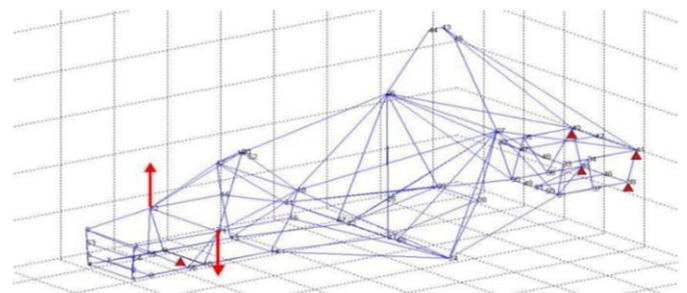
Figure 16. Frame Finite Element Model Loading Case [112]
