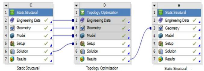
Figure 11. Structural analysis and topology optimization scheme [99]
