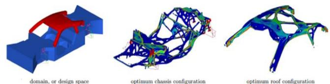
Figure 14. Automotive chassis topology optimization. In the results, the density ranges from 0.1 (blue) to 1.0 (red)
