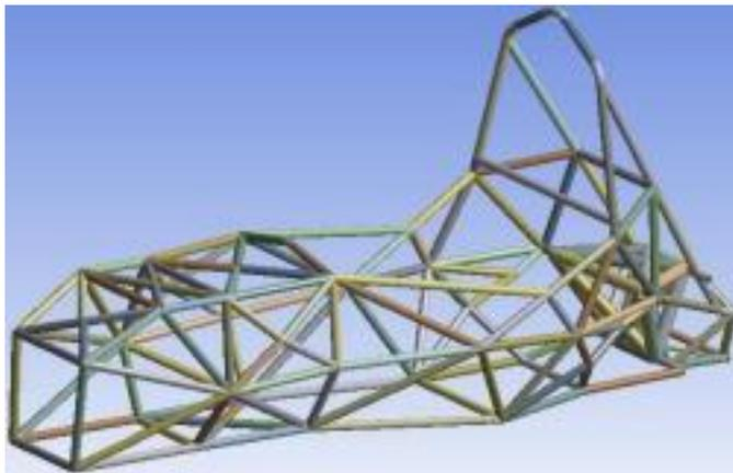
Figure 7. A complete model of a tubular space frame chassis [60]
