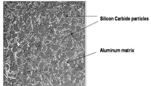
Figure 1. Microscopic structure of Al-SiC [30]
