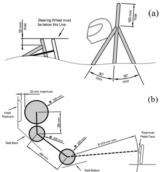
Figure 5. This figure shows the design of (a) main hoop and (b) driver position [71]
