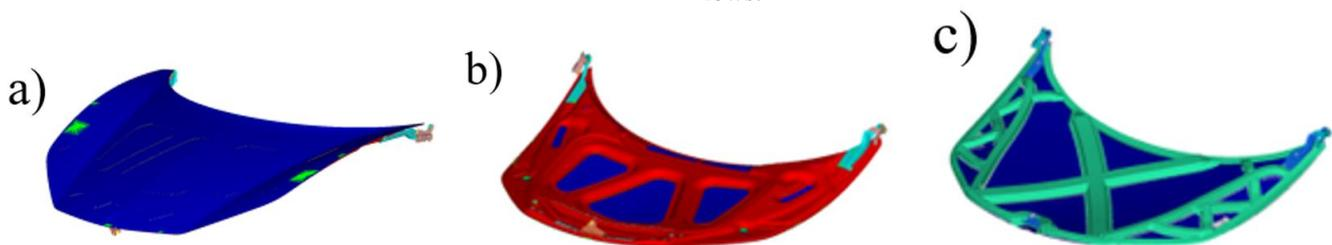
Figure 9. Reference model a) top view, b) side view, and c) optimum layout
