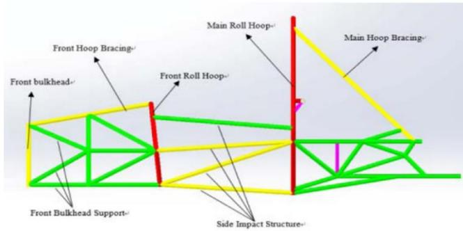
Figure 2. Showing the different parts of a chassis [65]
