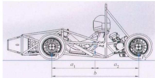
Figure 3. This figure shows the wheel base of the car [70]
