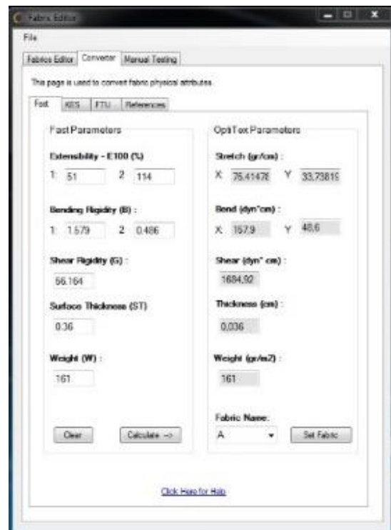
Figure 1. Fabric Editor converting the fabric parameters (showing the fabric parameters for Fabric code A).
