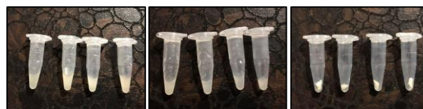
Fig. 1 The different ratio of waste cellulose: CMC based hydrogels (a), alcogels (b) and aerogel (c) after freeze-drying
