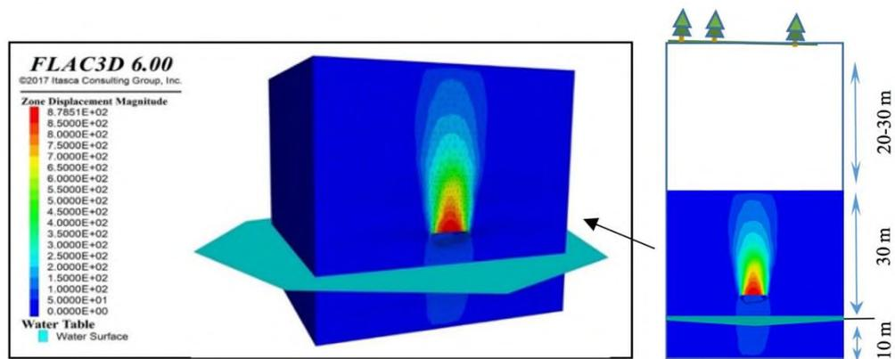
**Figure 13.** Induced displacement zone values (in mm) for the 2<sup>nd</sup> case scenario modelled through FLAC 3D for hypothetical small-scale roof cavity of groundwater conduit tending to develop sinkhole.
