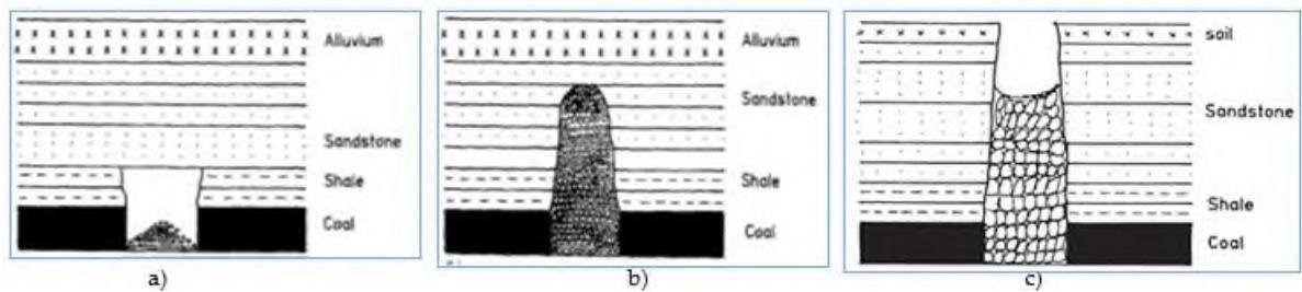
**Figure 5.** Rock mass collapse migration through overburden layers, [17].
