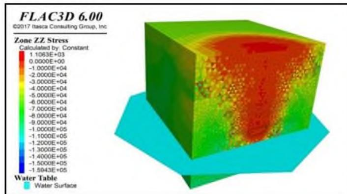
**Figure 14.** Induced vertical stress (in Pa) distributions for the 2<sup>nd</sup> case scenario at the modelled hypothetical sinkhole development through FLAC 3D start from small scale roof cavity of underground groundwater conduit tending to chimney type sinkhole.
