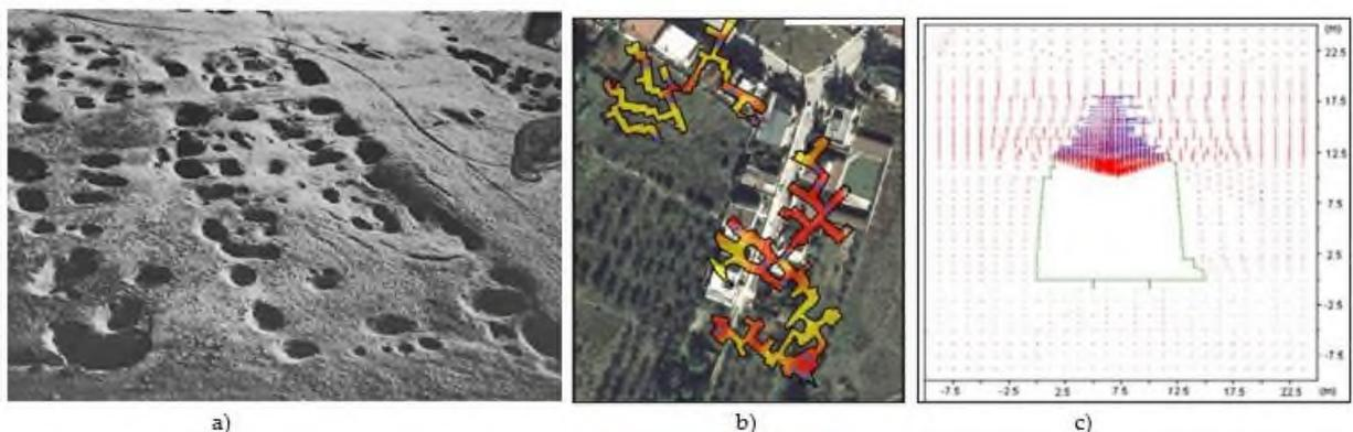
**Figure 4.** a) Ground surface deformations due to coal mine subsidence holes, troughs, and cracks above a coal mine at the Western Powder River Basin, Wyoming, US, (Photo-graph; C.R. Dunrud), [11], b) Location of instability evidences, (Barcelona Street, Altamura, Italy), [15], c) Example of numerical (distinct element method) analysis which helps to understand failure conditions around the underground mined out spaces at Castellana, Italy, [16].
