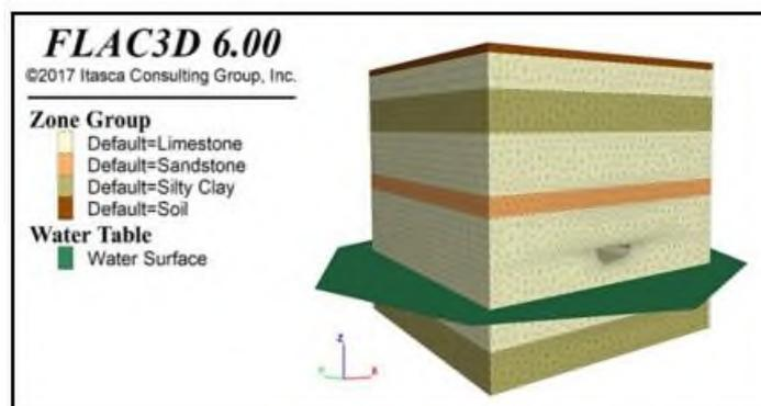
Figure 12. Hypothetical layered rock mass modelling example for the analysis of 2<sup>nd</sup> scenario through FLAC 3D analyses.
