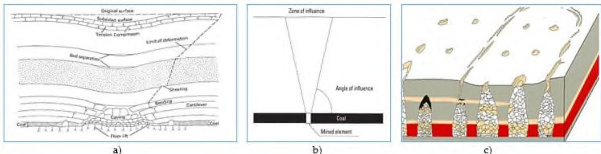
**Figure 3.** Subsidence influences, a) Deformations (caving) of overburden rock masses due to coal seam mining [11, modified from 12], b) Influence zone above coal seam galleries (or panels) which have tendency of caving (schematic illustration), [13], c) Collapses of over layer rock masses governed by induced stress conditions and rock mass discontinuities, [14].
