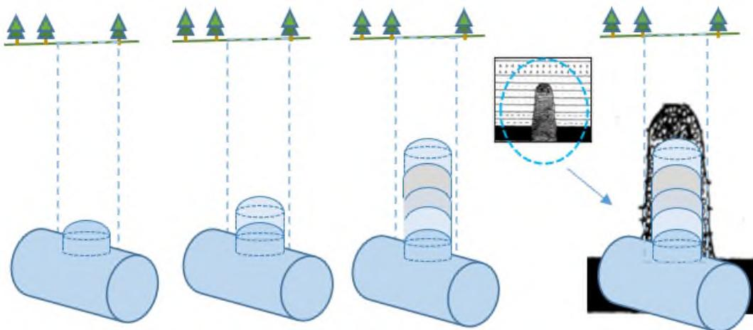
**Figure 9.** Hypothetical considerations for chimney type sinkhole development. Caving procedures have taken place in time step by step in upward direction where the rock masses are fractured according to induced 3D stresses-strains conditions.
