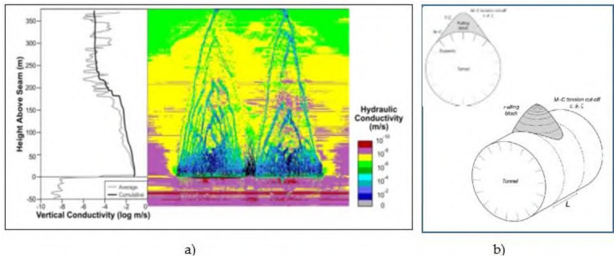
**Figure 6.** a) Rock masses hydraulic conductivity differentiation in modelled coal-seam overburden rock mass, [19], b) Triangular arch-shaped cavity considerations through Mohr-Coulomb (M-C) envelope & Tension-cut off (T-C), [21].
