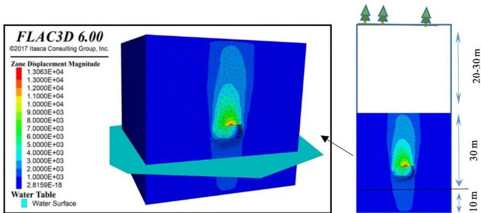
Figure 10. Induced displacement zone values (in mm) for the 1<sup>st</sup> case scenario modelled through FLAC 3D for hypothetical small scale roof cavity of groundwater conduit tending to develop sinkhole.
