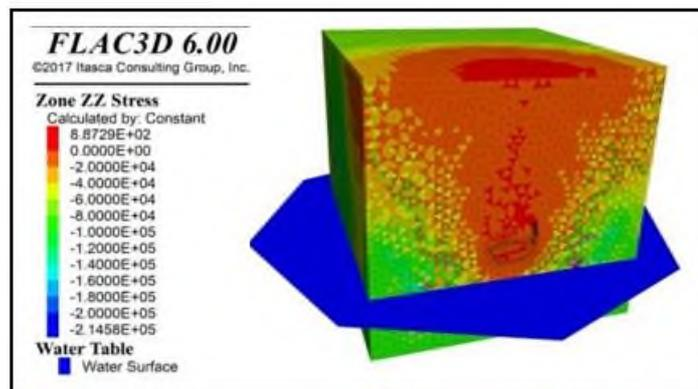
Figure 11. Induced vertical stress (in Pa) distributions for the 1<sup>st</sup> case scenario at the modelled hypothetical sinkhole development through FLAC 3D start from small scale roof cavity of groundwater conduit tending to chimney type sinkhole.
