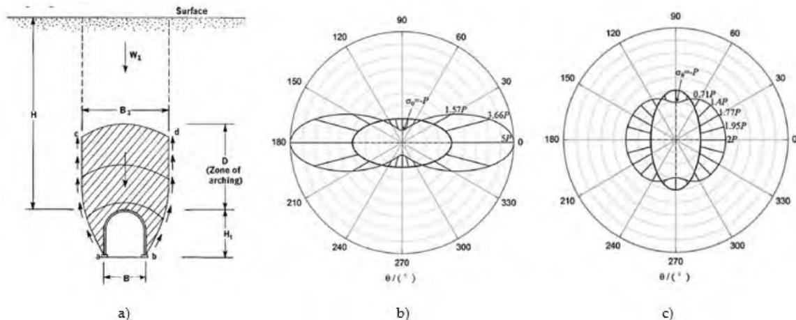
**Figure 2.** a) Rock-load height concept supplied by Terzaghi, [8], b) Induced tangential stresses around elliptical (long axis length=12mm, short axis length=10mm) holes with (b) horizontal (0°) and, (c) vertical (90°) inclination angle under uniaxial compression (P), [10].
