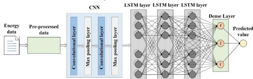
Figure 5. The structure of the created CNN-LSTM model
