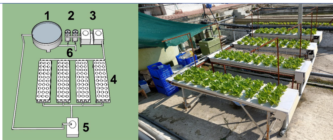
Figure 1. Nutrient film technique aquaponics 1: Fish tank, 2: Separation tanks, 3: Bio-filter, 4: Hydroponic unit, 5: Sump/Pump, 6: Sludge-water discharge pipe
