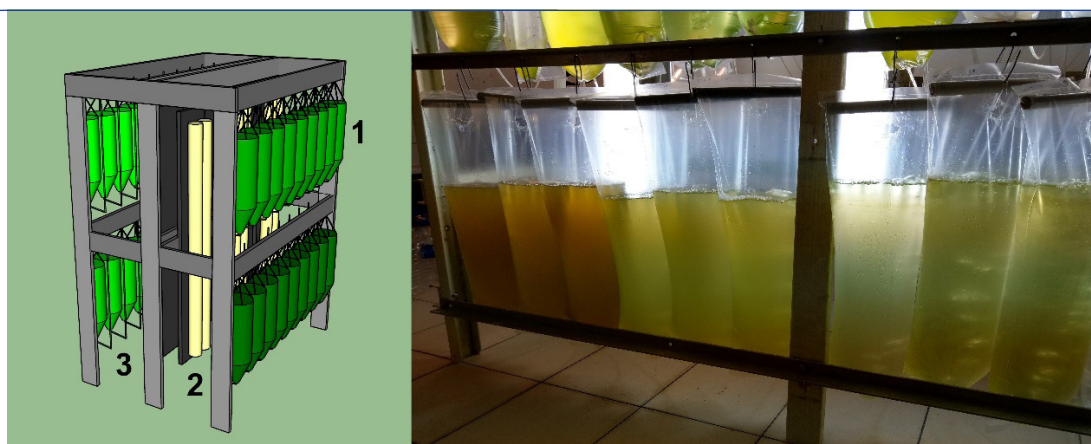
Figure 2. Microalgae batch culture platform 1: Polyethylene plastic bags with microalgae, 2: 36 Watt fluorescent lamps, 3: 2.5 \text{ L/min} aeration
