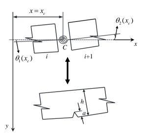
Figure 2. Cracked section represented by massless rotational spring.
