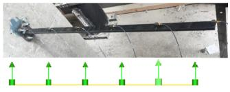
**Figure 4.** Laboratory model and accelerometer locations.
