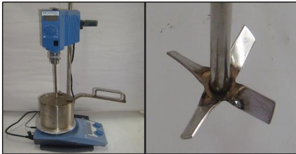
Fig 1. Modified bitumen mixer and mixing apparatus
