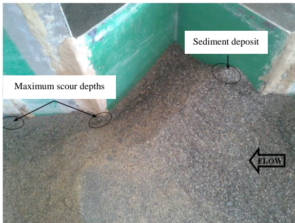
Figure 4. Sediment deposit and scouring observed in the present study.
