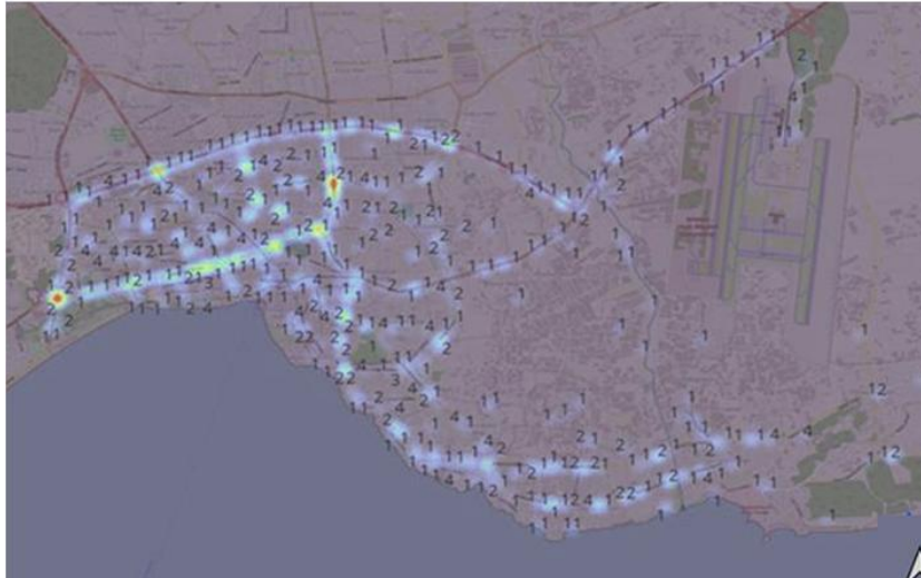
Figure 5. Accidents caused by insufficient stopping sight distance
