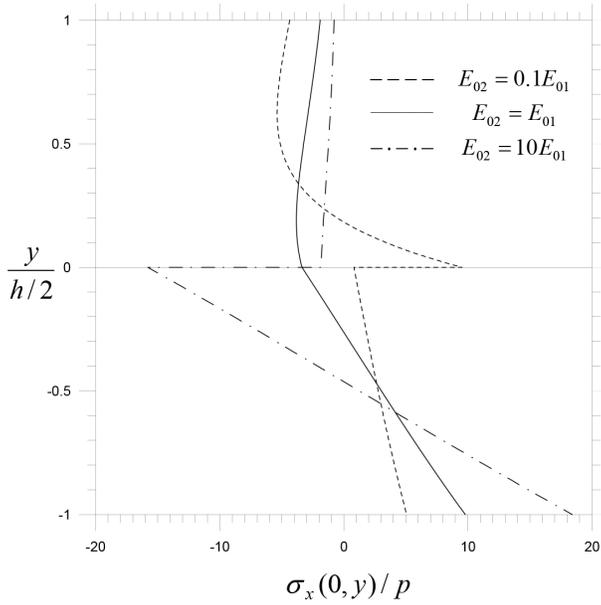
**Figure 7.** Axial stress  $\sigma_x(0, y)$  distribution along the thickness of the layered beam for various values of  $E_{02}/E_{01}$ , in the case of homogeneous lower layer. ( $h_1 = h_2$ ,  $h/L = 1/\pi$ ,  $E_{h1} = 0.1E_{01}$ ,  $E_{h2} = E_{02}$ ).
