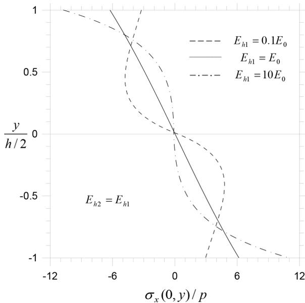
**Figure 5.** Axial stress  $\sigma_x(0, y)$  distribution along the thickness of the layered beam for various values of  $E_{hi}/E_0$ : variation of Young's modulus is symmetrical about the mid-plane, ( $h_1 = h_2$ ,  $h/L = 1/\pi$ ,  $E_{01} = E_{02} = E_0$ ).
