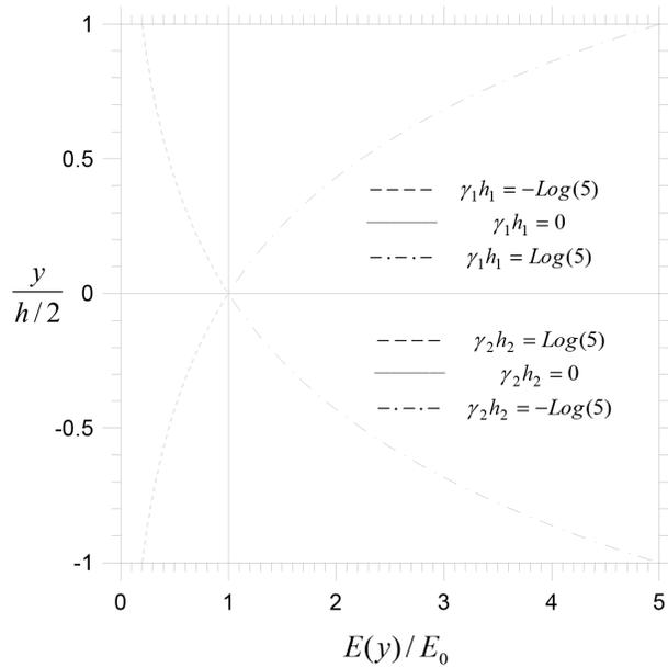
**Figure 2.** Variation of Young's moduli in the thickness direction, ( $h_1 = h_2, E_{01} = E_{02} = E_0$ ).
