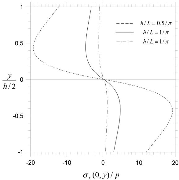
**Figure 9.** Axial stress  $\sigma_x(0, y)$  distribution along the thickness of the layered beam for various values of  $h/L$ , ( $h_1 = h_2$ ,  $E_{h1} = E_{h2} = 0.1E_0$ ).
