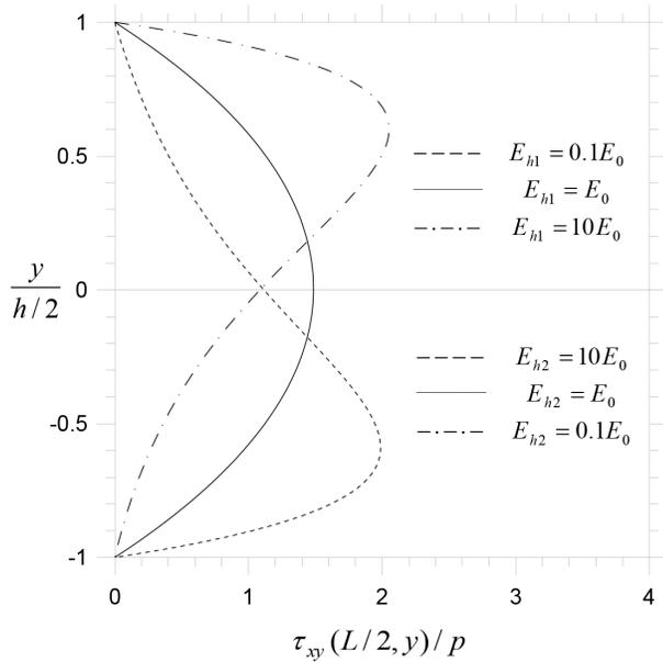
**Figure 4.** Transverse shear stress  $\tau_{xy}(L/2, y)$  distribution along the right face of the layered beam for various values of  $E_{hi}/E_0$ : variation of Young’s modulus is not symmetrical about the mid-plane, ( $h_1 = h_2, h/L = 1/\pi, E_{01} = E_{02} = E_0$ ).
