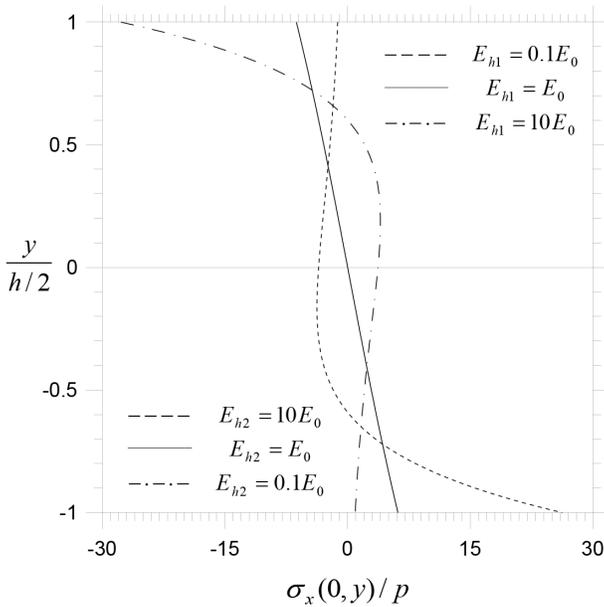
**Figure 3.** Axial stress  $\sigma_x(0, y)$  distribution along the thickness of the layered beam for various values of  $E_{hi}/E_0$ : variation of Young’s modulus is not symmetrical about the mid-plane, ( $h_1 = h_2, h/L = 1/\pi, E_{01} = E_{02} = E_0$ ).
