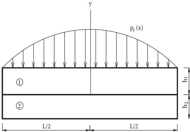
**Figure 1.** Geometry of a layered FG beam subjected to symmetric transverse loading.
