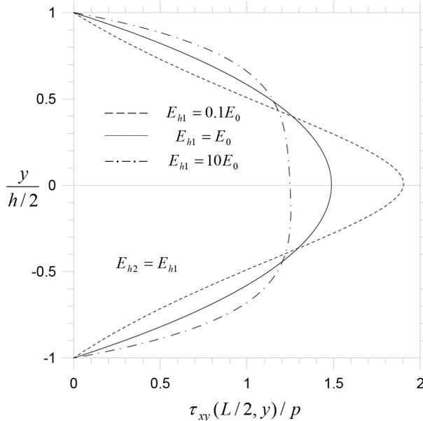
**Figure 6.** Transverse shear stress  $\tau_{xy}(L/2, y)$  distribution along the right face of the layered beam for various values of  $E_{hi}/E_0$ : variation of Young's modulus is symmetrical about the mid-plane. ( $h_1 = h_2$ ,  $h/L = 1/\pi$ ,  $E_{01} = E_{02} = E_0$ ).
