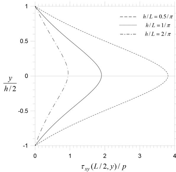
**Figure 10.** Transverse shear stress  $\tau_{xy}(L/2, y)$  distribution along the right face of the layered beam for various values of  $h/L$ . ( $h_1 = h_2$ ,  $E_{h1} = E_{h2} = 0.1E_0$ ).
