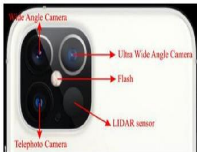
Figure 1. Iphone 14 pro camera and sensor system [13]
