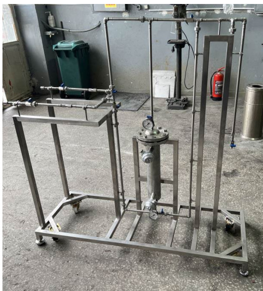
Figure 2. The production version of lab scale PSA experimental setup
