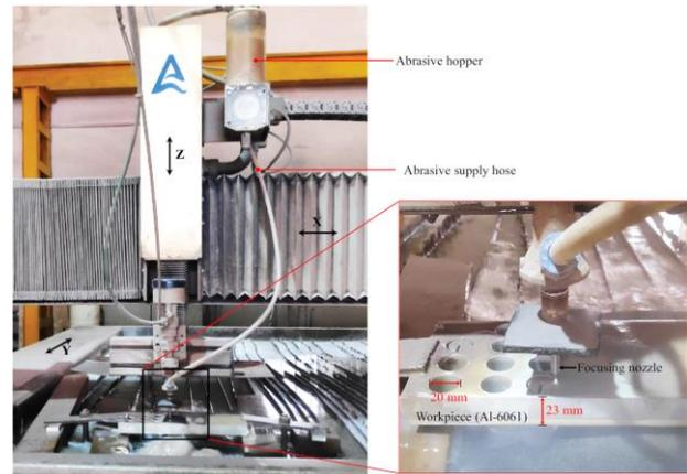
Figure 1. Experimental setup employed for AWJ trepanning [1].
