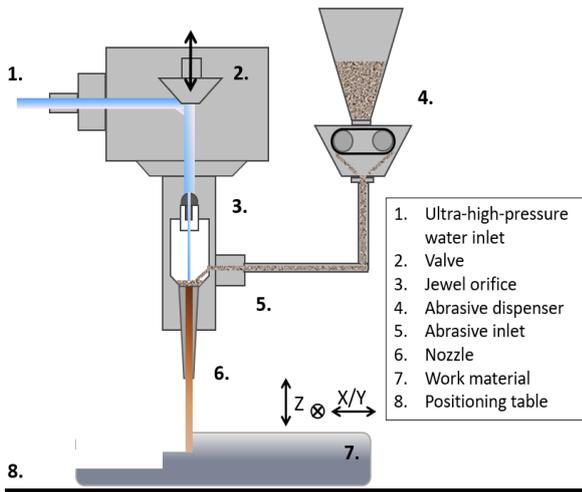
Figure 4. Schematic overview of the AWJ components [5].
