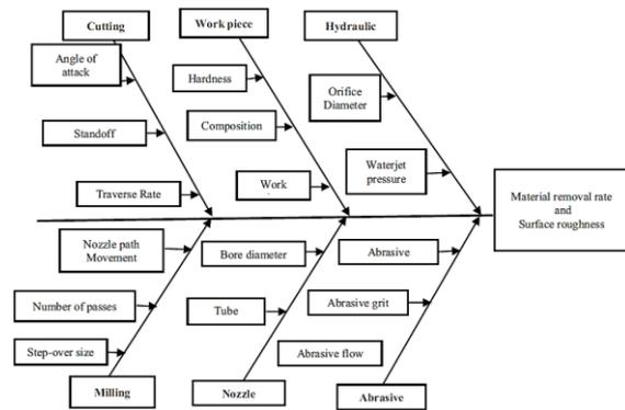
Figure 8. Process parameters involved in AWJ milling [13].
