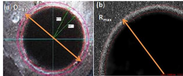
Figure 6. Measurement of maximum damage drilled hole diameter ( $D_{max}$ ): (a) Peel up at the entry hole and (b) Push out at the exit hole [8].
