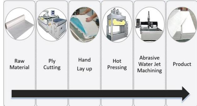
Figure 5. UHMWPE plate production flow chart [7].
