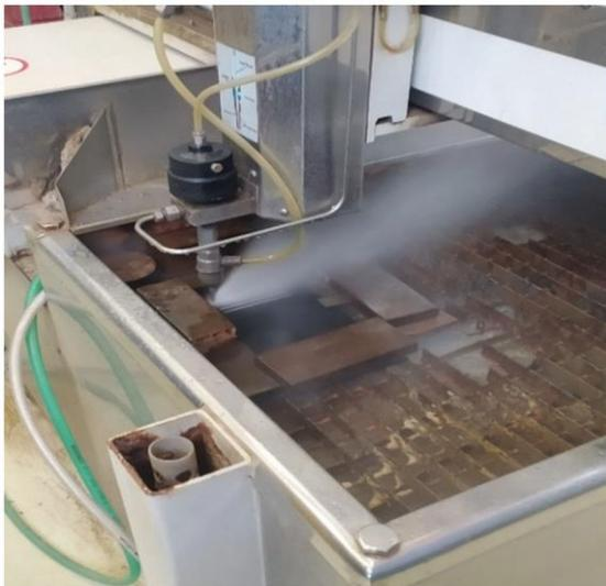
Figure 12. AWAC CNC waterjet cutting machine AWJ CT 0806: waterjet cutting process [67].
