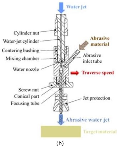
Figure 7. Principle of AWJ machining: (a) process parameters (b) components of cutting head [12].
