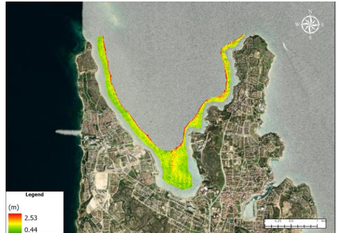
Figure 10. Spatial distribution of differences between multi beam bathymetry and UAV-based DEM
