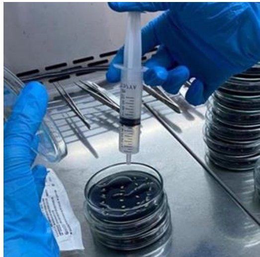
Figure 3. Adding filter-sterilized colchicine onto anthers for biphasic applications
