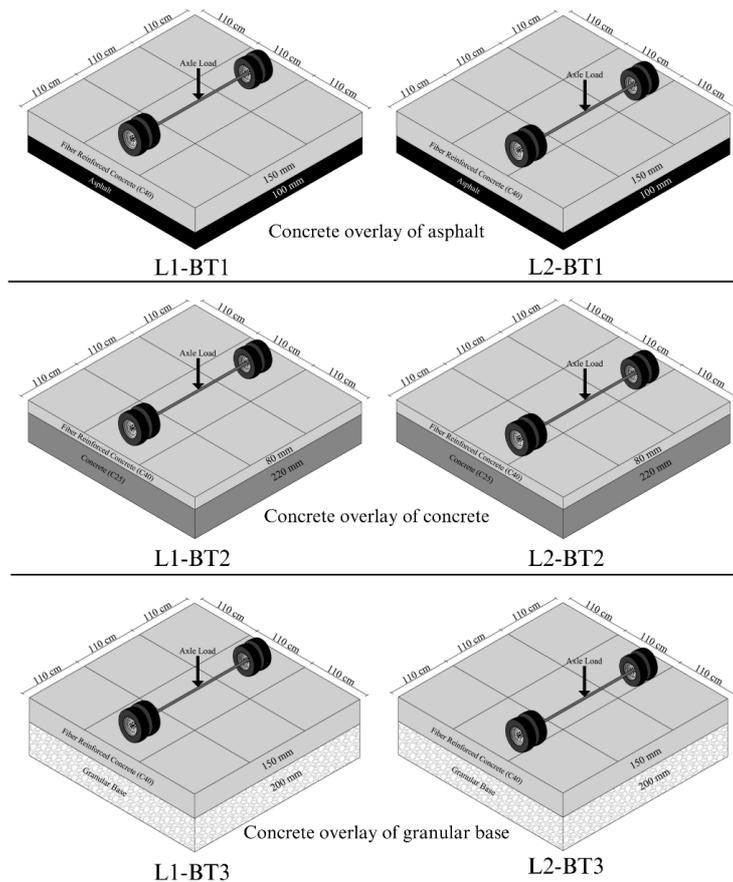
Fig. 5. Loading position and pavement structure combinations
