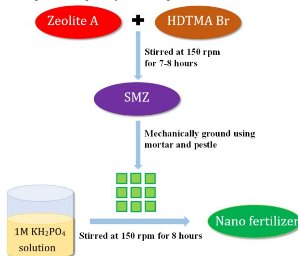
Figure 1. Schematic representation of preparation of Zeolite based nano P fertilizer
