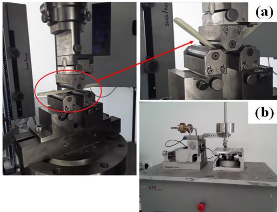
Figure 4. a) Zwick Roell flexural strength tester and b) UTS Tribometer T10/20 wear tester device
