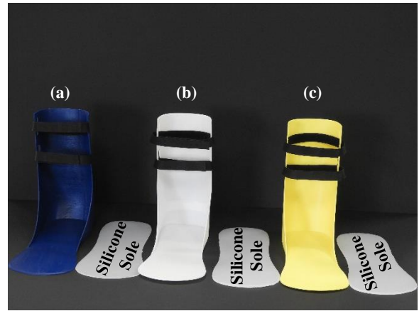
Figure 3. AFOs with (a) TPU, (b) HIPS, and (c) PLA materials, featuring silicone sole
