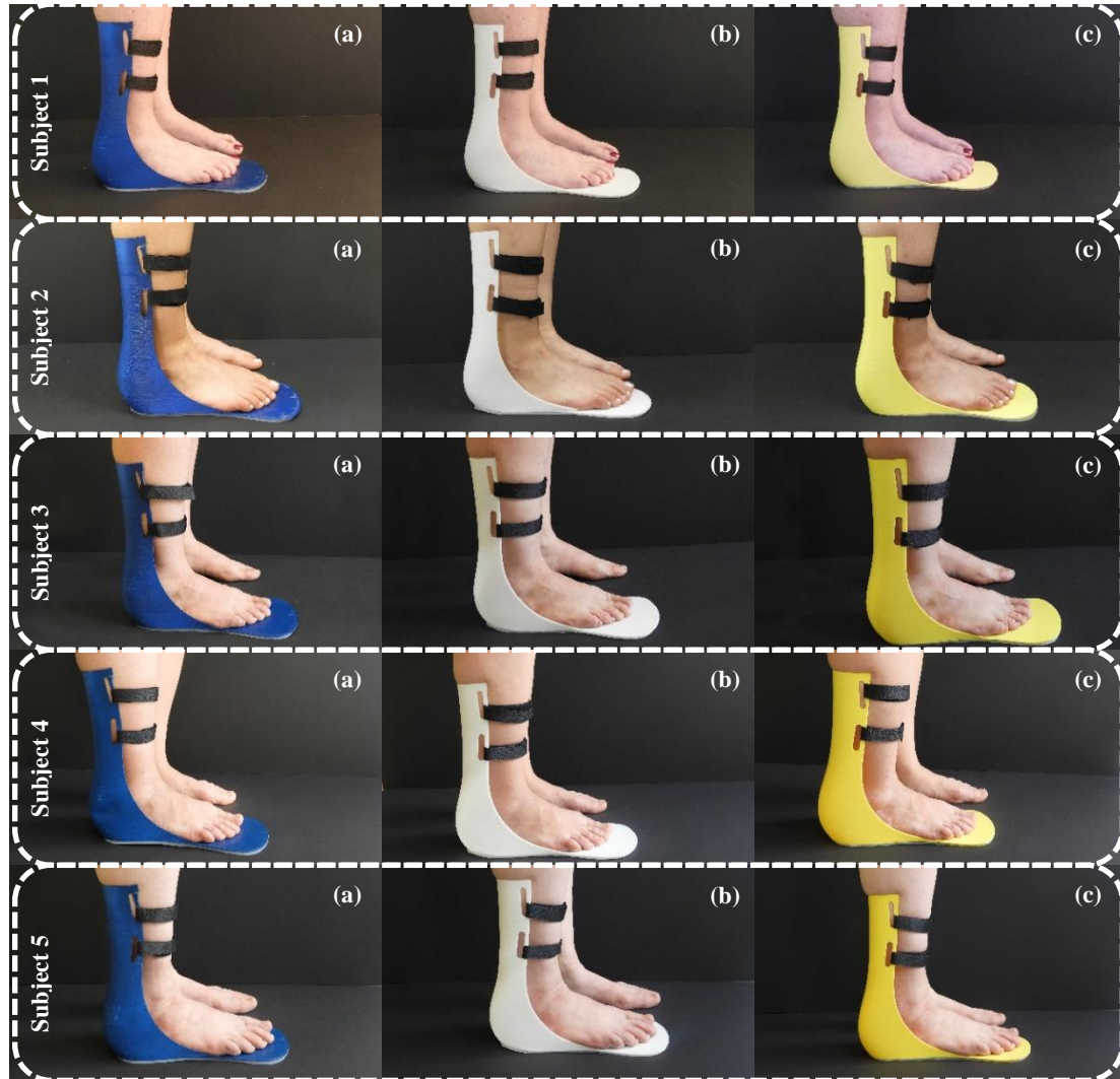
Figure 6. AFOs experienced by the subjects: (a) TPU, (b) HIPS, and (c) PLA
