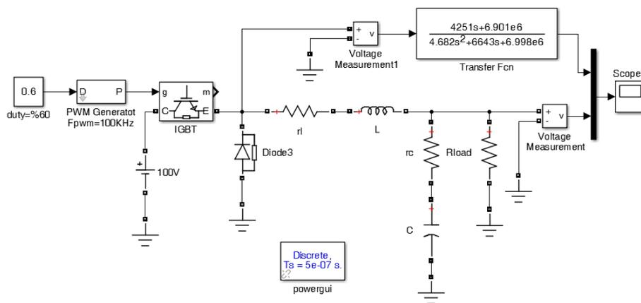
Figure 3. Simulation platform for T(s)'s accuracy test
