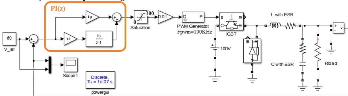
Figure 5. PI(z) based Buck converter control block diagram
