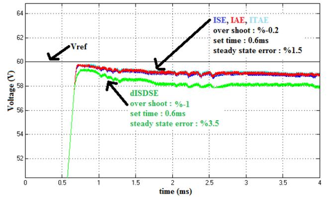
Figure 11. Control results for 4 different Kp and Ki parameters
