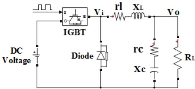
Figure 2. Buck converter topology
