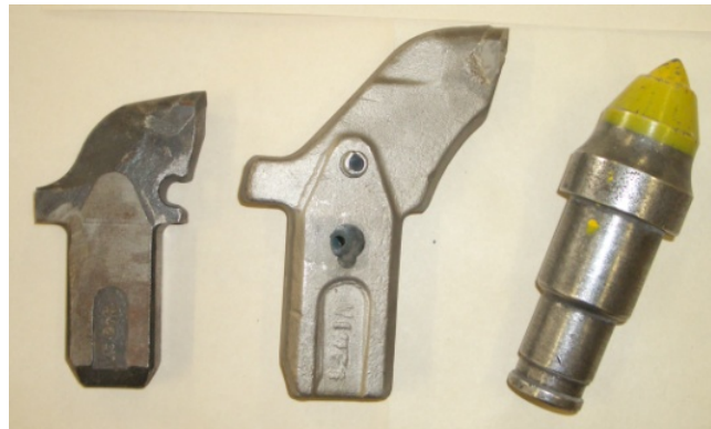
Figure 1. Radial, Forward-Attack and Point-Attack Picks
