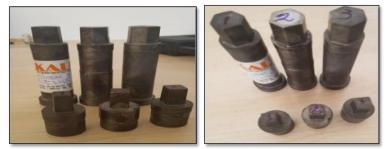
Figure 2. The types of three punch sets (Üçlü zımba setleri)
