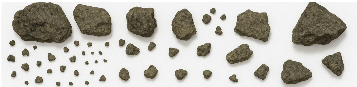
Figure 3. Surface image of a typical steel slag aggregates
