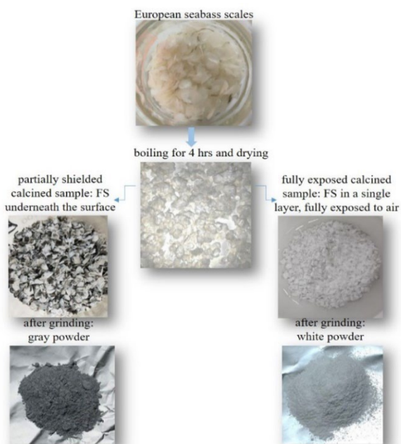
Figure 1. Schematic representation of hydroxyapatite (HAp) powder preparation from European seabass scales. The top image shows the cleaned fish scales after removing dirt and debris. The central image depicts the scales after boiling for 4 hours and drying in a fume hood for 24 hours. The left image shows the gray powder obtained from partially shielded scales, where inner scales were shielded from air exposure during calcination. On the right is the white powder, derived from fully exposed scales calcined in a single layer, allowing full air exposure. The bottom images show the final powders after grinding, highlighting the distinct color differences between the gray and white powders
