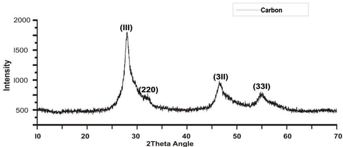
Figure 5. XRD pattern of 40 g carbon nanomaterial.
