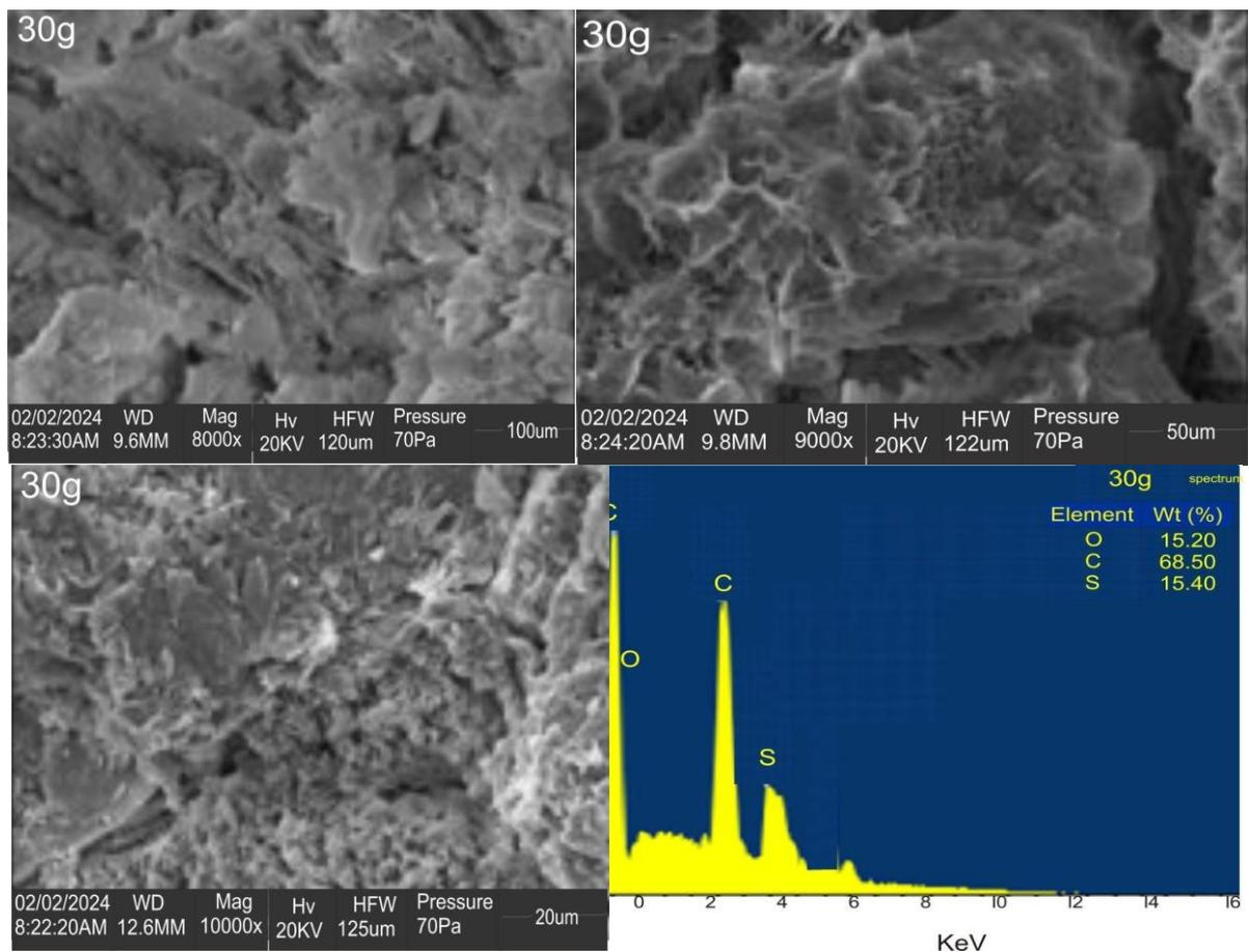
Figure 3. SEM Photograph of 30 g carbon nanoparticle with variation of glucose of a) 20  $\mu\text{m}$  M, b) 50  $\mu\text{m}$ , c) 100 $\mu\text{m}$  and d) EDX.
