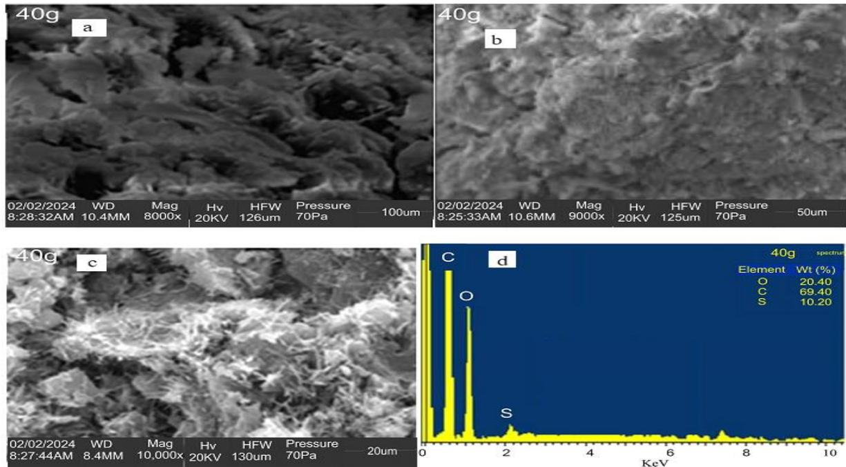
Figure 2. SEM Photograph of 40 g carbon nanoparticle with variation of glucose of a) 20  $\mu\text{m}$  b) 50  $\mu\text{m}$ , c) 100 $\mu\text{m}$  and d) EDX.
