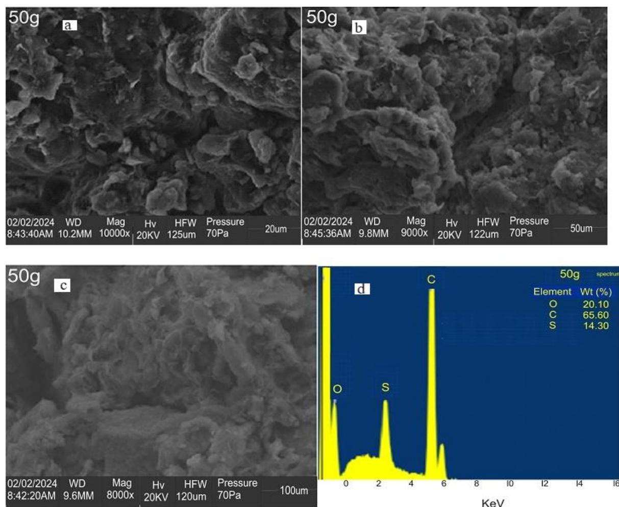
Figure 1. SEM Photograph of 50 g carbon nanoparticle with variation of glucose of a) 20 µm M, b) 50 µm, c) 100µm and d) EDX.
