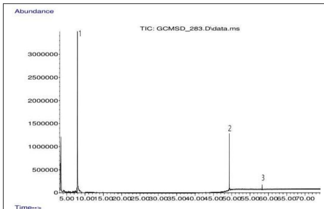
**Figure 12.** Chromatograms of beans sample spiked with mixed standard of dichlorvos and bifenthrin1: Dichlorvos2: Triphenylphosphate3.
