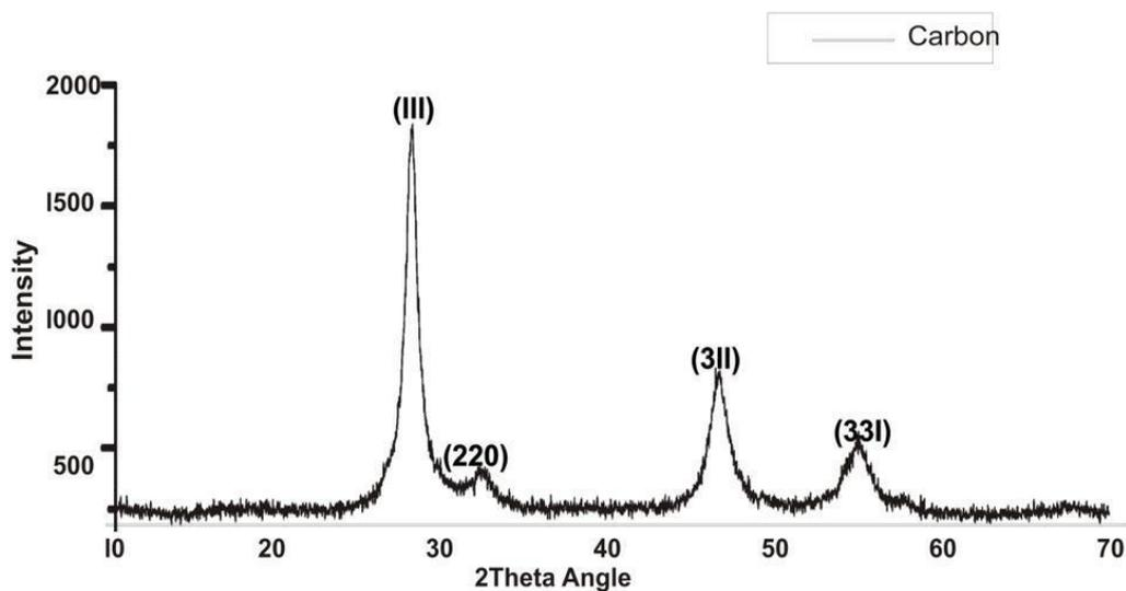
Figure 6. XRD pattern of 50 g carbon nanomaterial.
