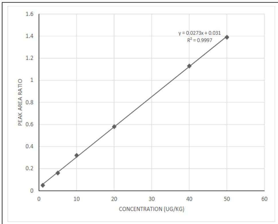
Figure 10. Calibration Curve for Bifenthrin.
