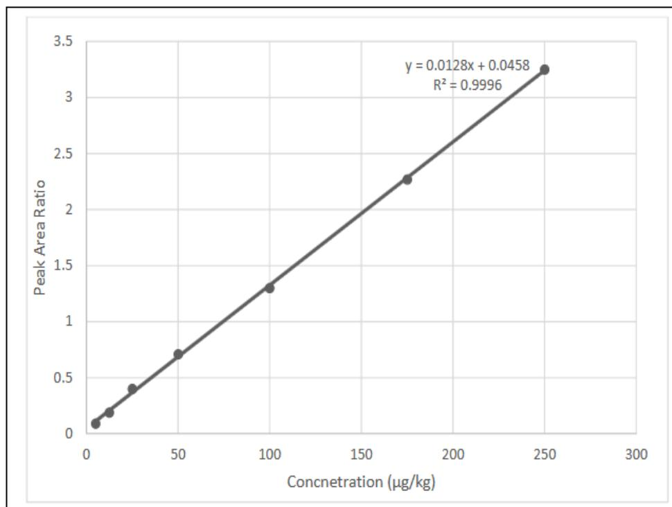
Figure 11. Calibration Curve for Dichlorvos.
