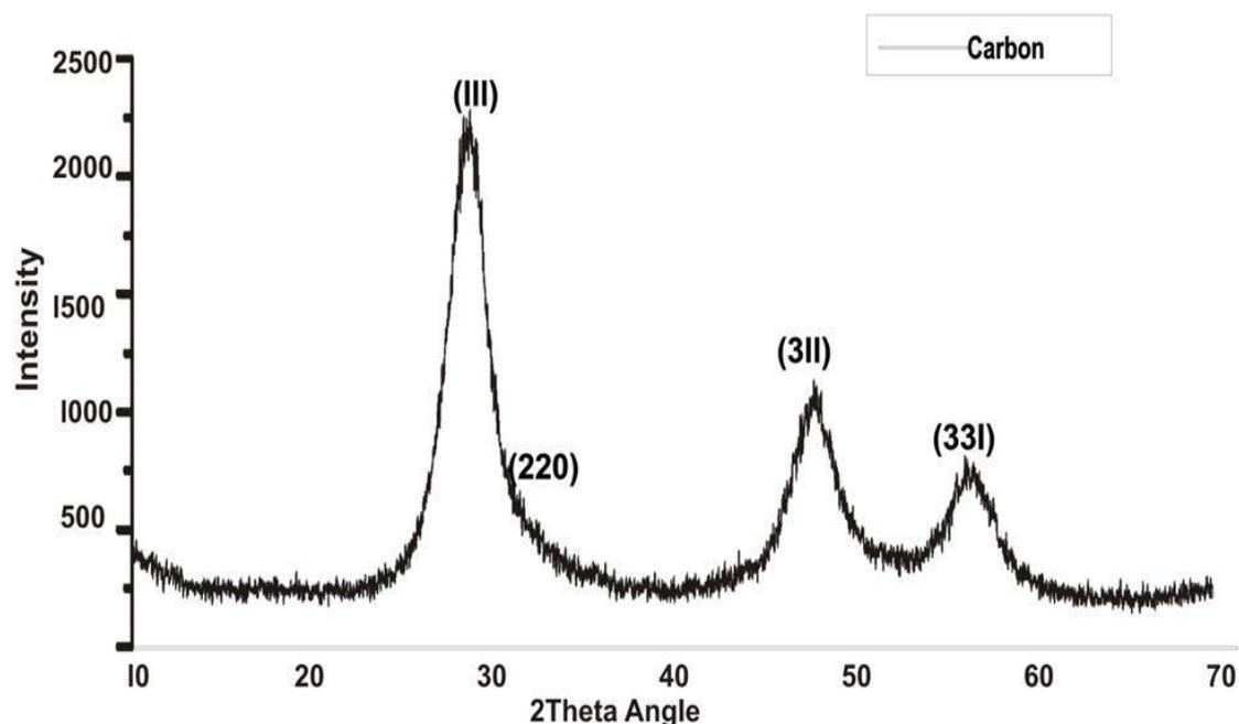
**Figure 4.** XRD pattern of 30 g carbon nanomaterial.
