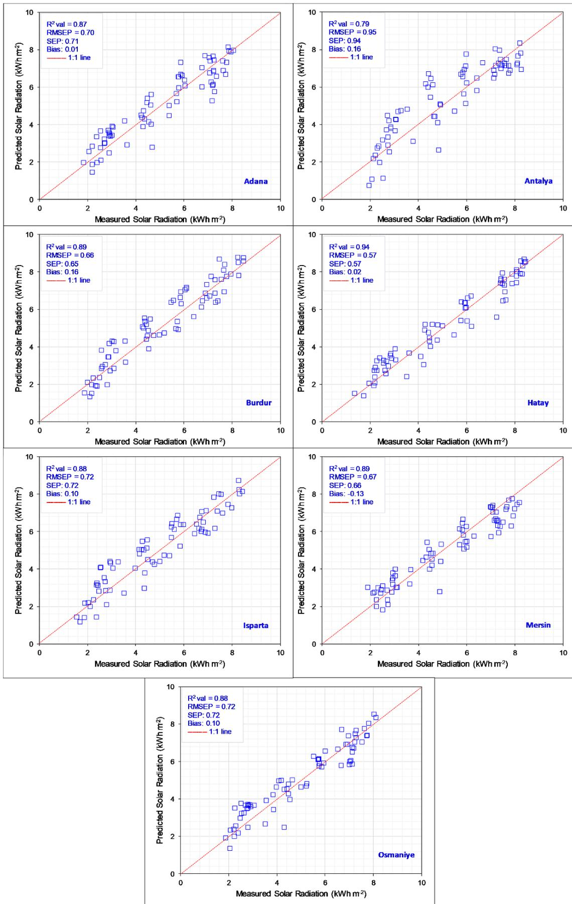
Fig. 2. Scatter plots of monthly average daily global solar radiation predictions obtained for each station for the test period.
