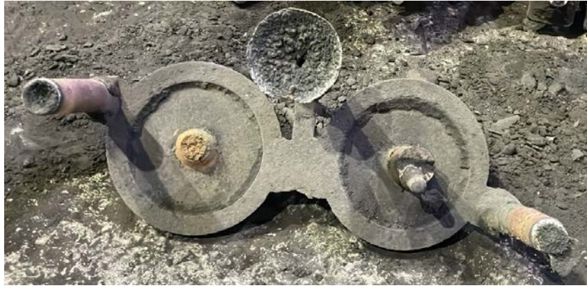
Figure 5. Trial production where casting simulations were verified
