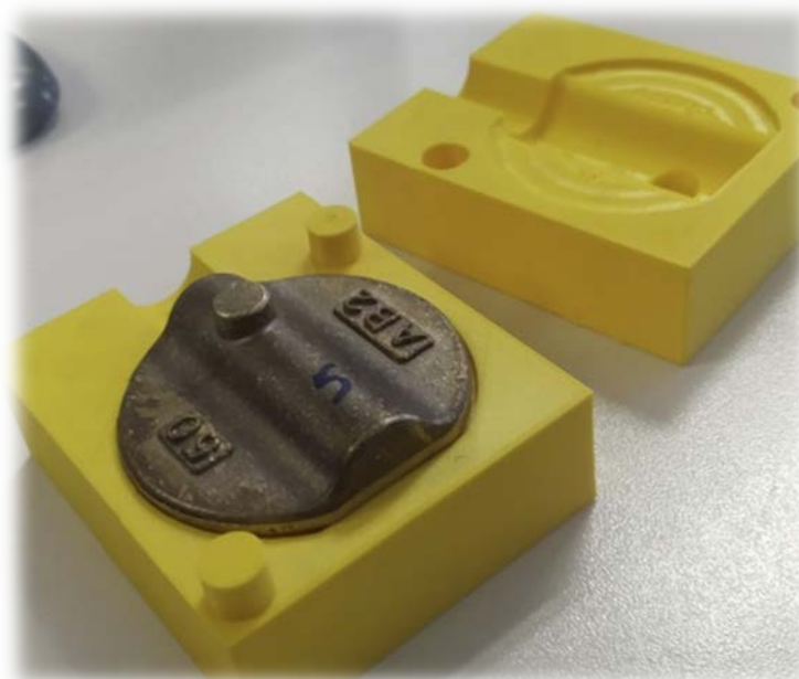
Figure 12. Core disc prototype production
