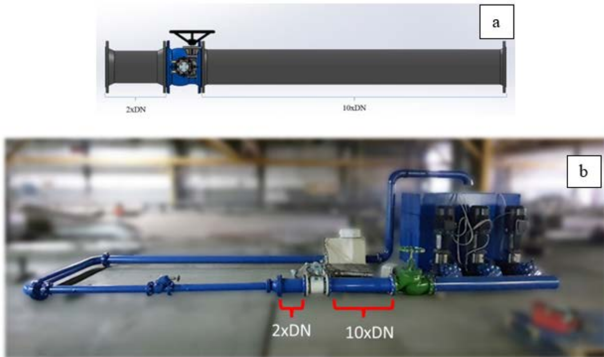
Figure 20. Test model (a) and field application (b)
