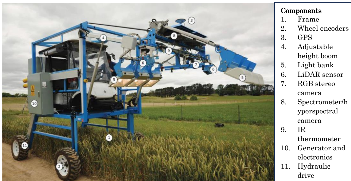
Figure 6. Advanced HTP system with sensor integration (Deery et al. , 2014).
